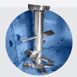
The primary mixing element of all Lancaster Products K-Series mixers is the single piece counter-rotating high-speed rotor. The design of the mixing rotor will vary depending upon the particular process requirements.
