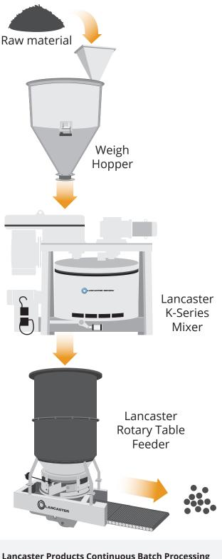
Lancaster Products Continuous Batch Processing System offers the benefits of both steady state throughput and product consistency. Materials leaving the rotary table feeder can continue to downstream processing or for final product bagging. The Lancaster Products Continuous Batch Processing (system) design enjoys the benefits of both continuous and batch processing.
